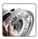
3) To install the Bona Power Drive drive plate, place the drive plate into position and turn it to engage the interlock *(C)*. Once it is in place, turn the small flat paddle lever *(D)* to make sure that it is bolted into place.
