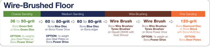
\*When a softer brushing effect is desired, use the Tynex Brush after wire-brushing.
