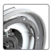
**4)** To remove the Bona Power Drive drive plate, turn the paddle lever so it is in the unlocked position *(E)*. Place the tip of the supplied box spanner between the driving axle and drive plate bracket, then push against the drive plate to release the interlock *(F)*. Turn one of the sanding discs counterclockwise until the drive plate can be freed.
