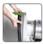
Always remove the dust skirt, extra weights, and the drive plate or sanding discs before transportation. Always vacuum and clean machine after use. When transporting the machine via vehicle, make sure that the machine is securely fastened through the wheels to avoid movement.
